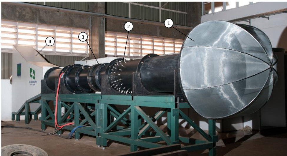
Fig. 1 Photograph of EESC-USP Fan Noise Test Rig setup showing ① inlet, ② microphone array, ③ fan-stator section, ④ exhaust.
