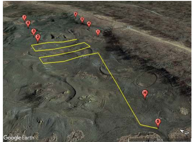
Fig. 4: The mission planning. Before the experiment, the operator selected 8 waypoints (marked 1 to 8) from Google Earth and saved them in a file. Once the operator gets to the experiment location (ash pit), using the drone itself, a position is selected for the base station (S) from where the drone is initially launched, and for the home position (H), which is close to the base and where the drone can land safely and the battery can be replaced.
