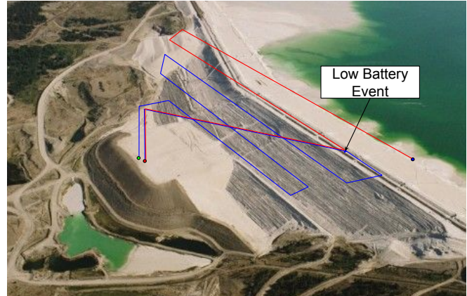
Fig. 1: Example of an inspection mission in a large tailing dam (used to store waste byproducts of mining). The drone takes off at the green dot with a mission defined by a lawnmower pattern path, which would lead to the blue dot when complete. However, since the mission given by the user was too long for the battery capacity, a low-battery event happened. The drone decides to return to its home position and land. After the battery was replaced, the drone resumed the mission from the point it was interrupted. The blue path was followed before the low battery event and the red path after the battery was replaced.
