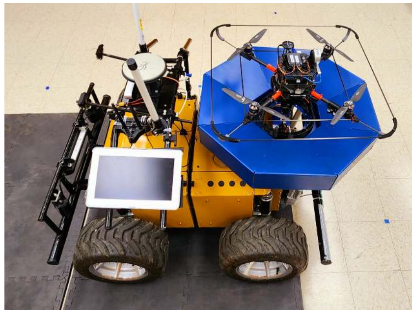
Figure 1. Rhino, the unmanned ground vehicle (UGV), is a mobile robot in yellow and blue. Oxpecker, the tethered unmanned aerial vehicle (TUAV), is the drone in black on top of the blue platform. Rhino and Oxpecker form a cooperative robotic system for underground mine mapping.
