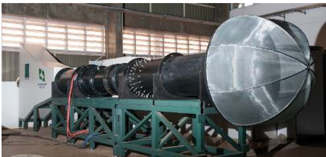
Fig. 1 The EESC-USP Fan Rig, an aeroacoustic wind tunnel for fan noise measurements.
