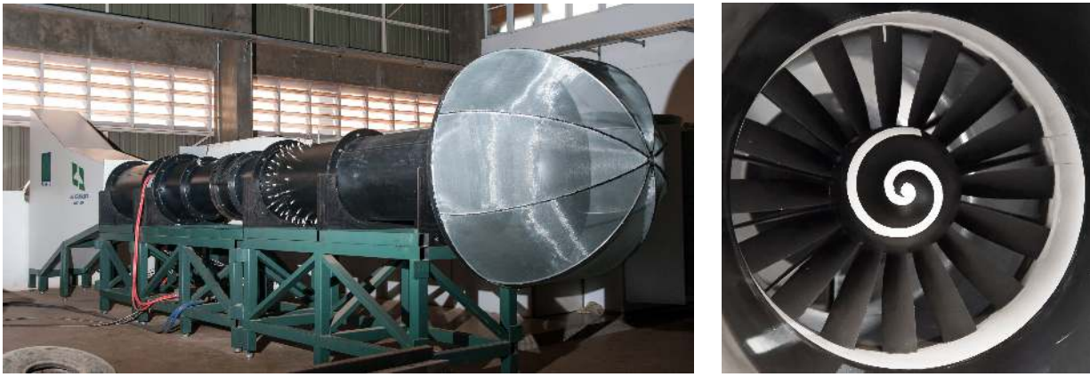
Figure 1. Left: Current EESC-USP Fan Rig setup. Right: 16-bladed fan close up.
