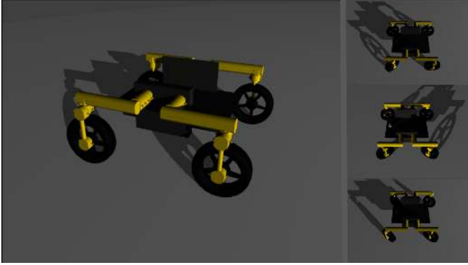
Fig. 2. The mobile platform, MoonTamer , is generated for testing the algorithms in the simulation environment. MoonTamer is a 4WD rover and able to perform skid-steering, Ackermann steering, omni-directional, and crab-walk motion.
